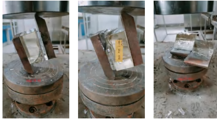
Figure 15 Shear Failure State of the Specimens
