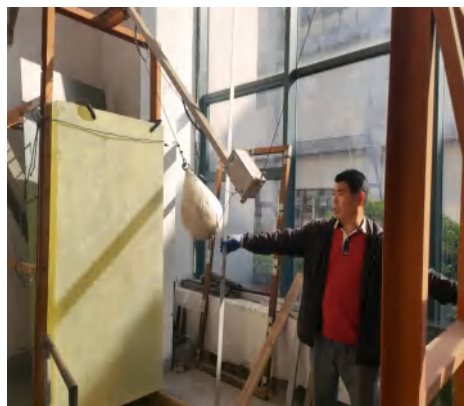
Figure 18 Pummel Bag Impact Test
