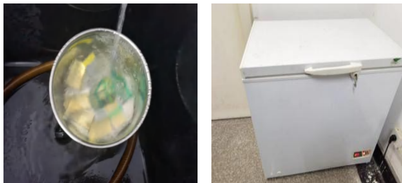
Figure 16 Freeze-Thaw Resistance Test of Specimens
