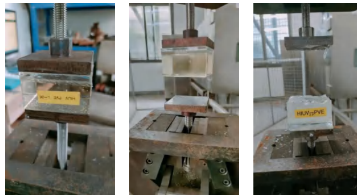
Figure 14 Flatwise Tension Bond Strength Test
