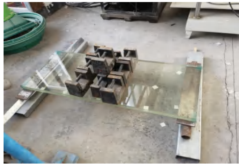
Figure 10 Static Bending Load Test
