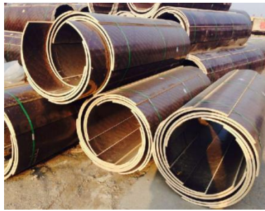
Figure 5 Circular Column Formwork
