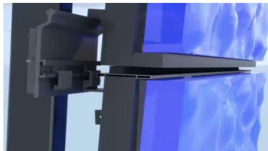
Figure 7 Virtual Pre-Assembly of LIULI Composite Curtain Wall Units
