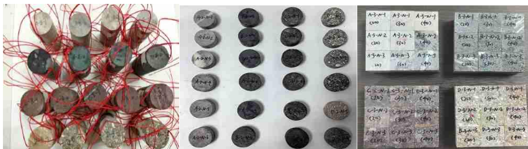
Figure 2 Machined Standard Test Specimens: (a) Standard Uniaxial Compression Specimen; (b) Standard Brazilian Disc Specimen; (c) Standard Variable-Angle Shear Specimen
