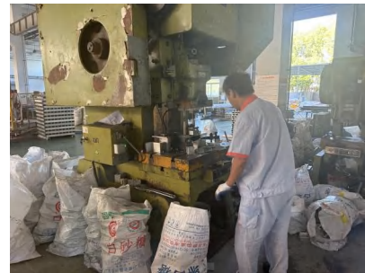
(b) Stamping of the Stainless Steel Hanging-Ear Connector
