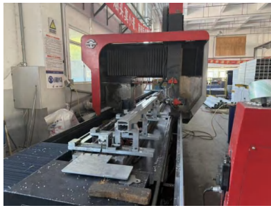
(a) Stamping of the Aluminum Profile Frame
