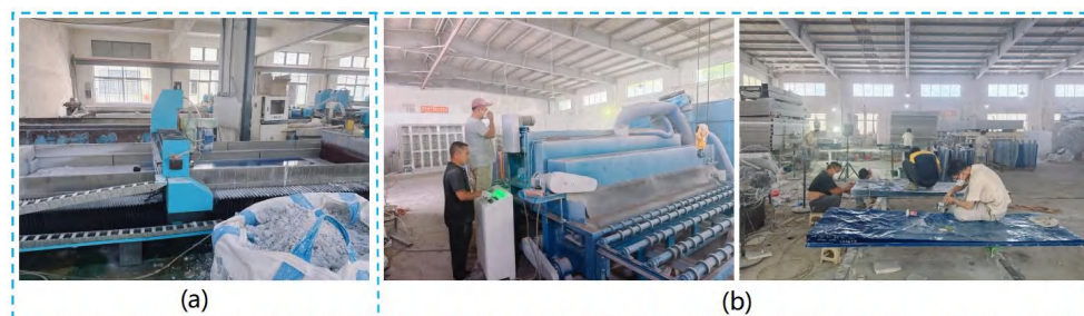
Figure 11 Machine Grinding Back Surface and Fine Grinding Corrugated Surface (a) Machine Grinding Back Surface; (b) Fine Grinding Corrugated Surface
