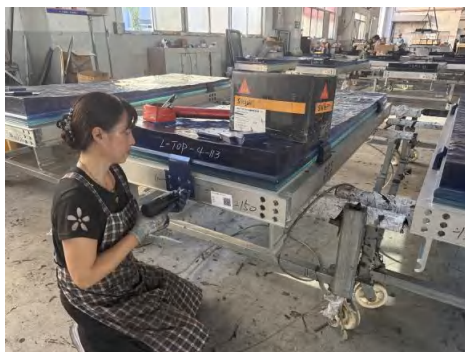
(a) Installation of Stainless Steel Edge Protectors
