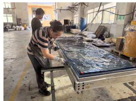
(b) Structural Sealant Application
