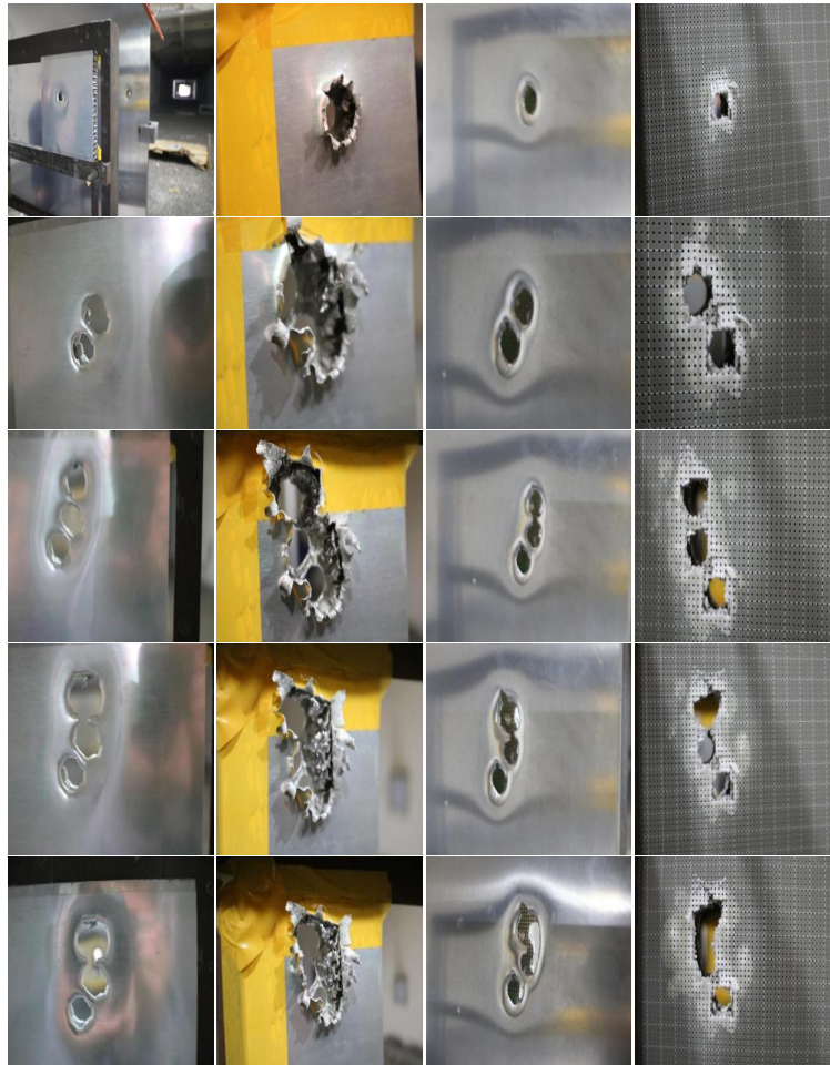
Figure 20 The Appearance of a Target Board (Columns from Left to Right: Honeycomb Aluminum Front Panel; Honeycomb Aluminum Rear Panel; Target of Aluminum Front Panel; Honeycomb Sandwich. Rows from Top to Bottom: Round 1 to Round 5)
