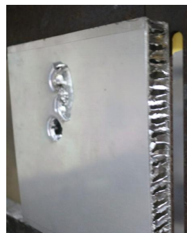
Figure 21 Damage Visible on the Rear of the Aluminum Honeycomb Plate
